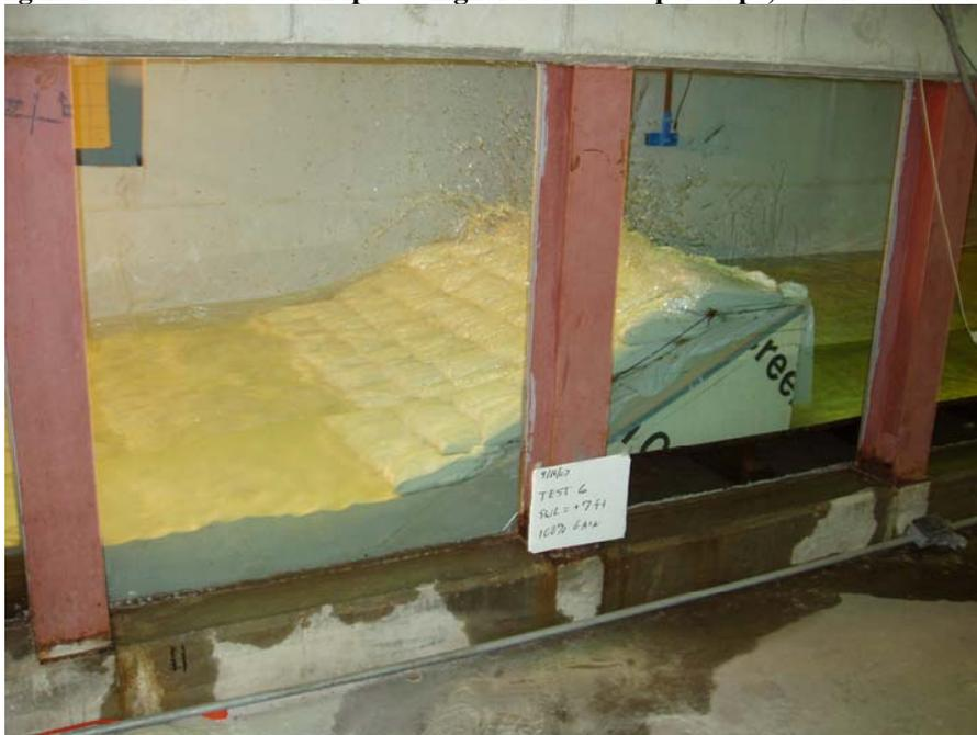
**Figure 19 Photo from 2007 USACE Laboratory Sandbag Revetment testing.**
